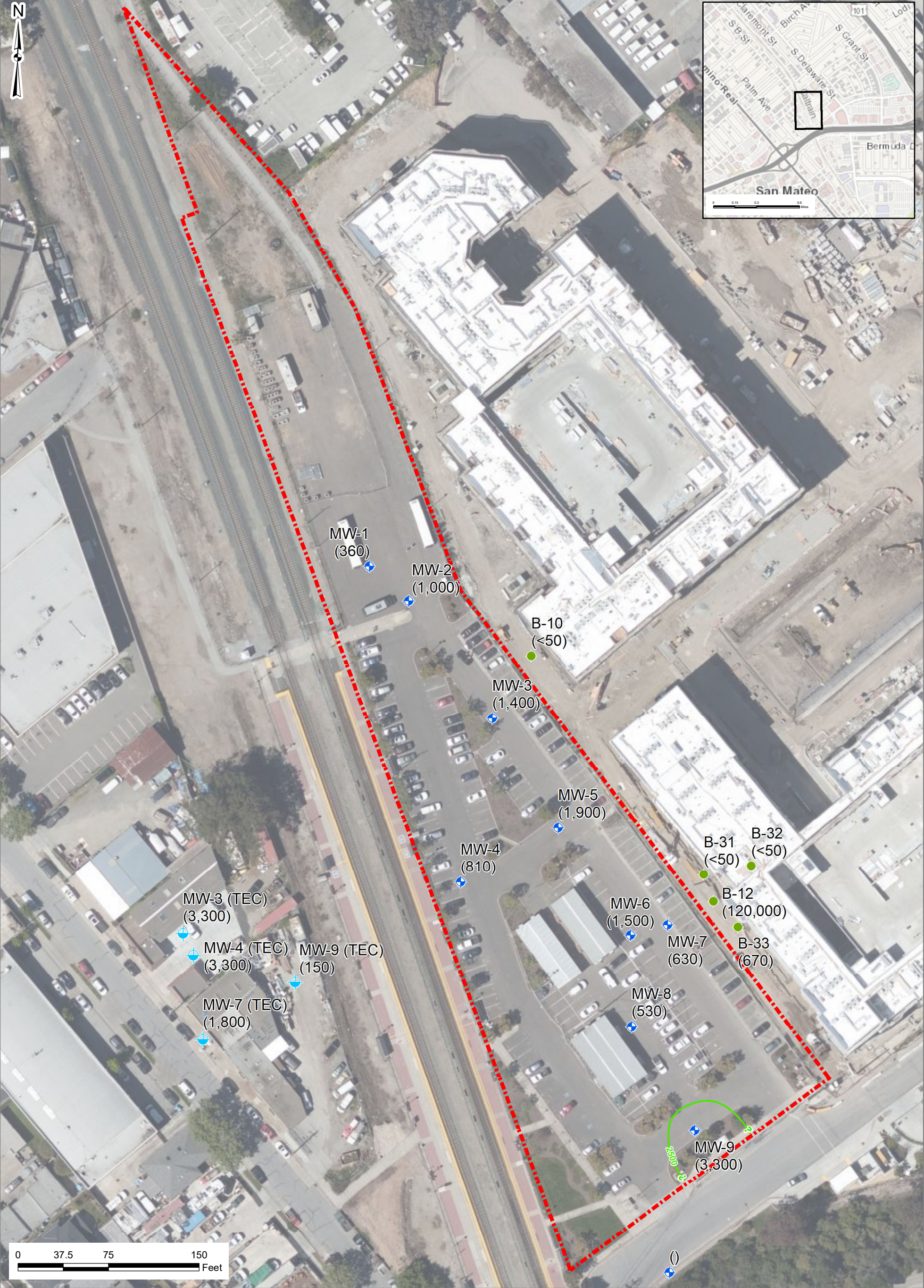
Legend Monitoring Well - ERM 2021 Groundwater Sample - Station Park Green Monitoring Well - TEC TPH-Diesel Isoconcentration, Dashed where Inferred, Queried where Uncertain Site Boundary Figure 12 TPH-Diesel Isoconcentration in Groundwater Hayward Park Caltrain Station San Mateo, California Environmental Resources Management www.erm.com
