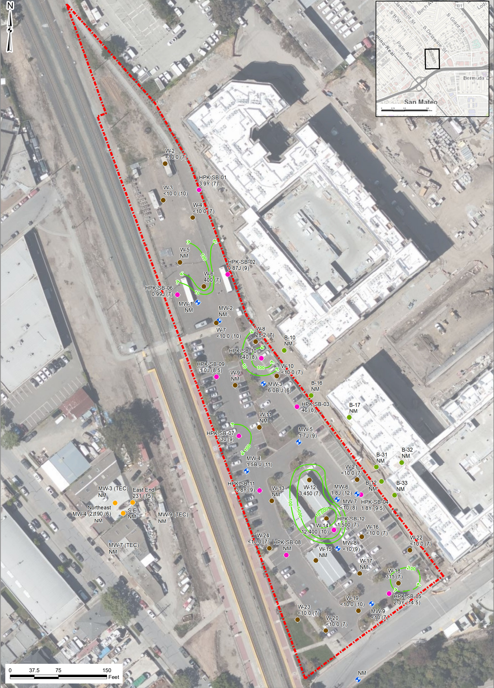
Figure 7 TPH-Diesel Soil Isoconcentration 6 to 11 ft bgs Hayward Park Caltrain Station San Mateo, California
